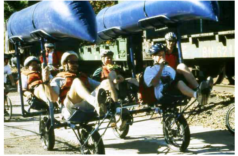
Four people on four wheels—good stability and high power-to-weight ratio.
