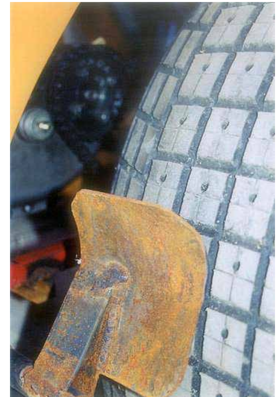
Basically just a lever that rubs on the tire, stage coach style, works well.
