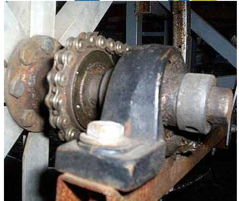
The big Omega shaped lump with the bolt thru the front of it, is a pillow block bearing. The other bolt is on the other "leg" of the Omega.
