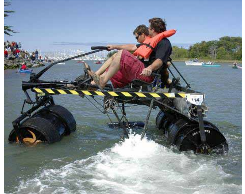
Drum Roll travels sideways in the water, minimizing the water resistance of the wheels/pontoons, and eliminating the angle drive for the propeller. Dig that prop wash!
